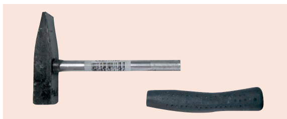
Figure 15: RAPEX notification no. 0125/06 deals with a hammer where the handle breaks.
