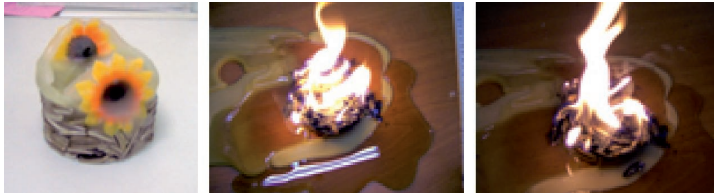
Figure 31: Candles containing plant parts may burn intensely with high flames and cause fires.
